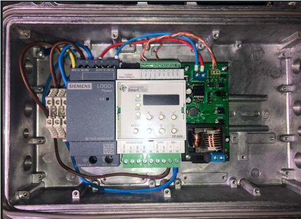
► The inside of an EMF generator assembled with a module controlled via the Internet
